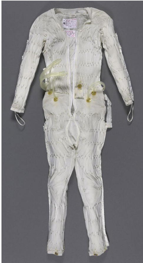
Figure 5. Liquid Cooling and Ventilation Garment (LCVG). Source: Smithsonian National Air and Space Museum, 2012
