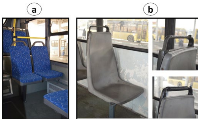
Figure 3. Comparison of two different bus seats in terms of vandalism signs (Authors).
